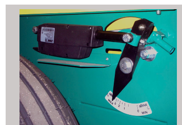
Electro hydraulic cylinder for adjusting flow rate
