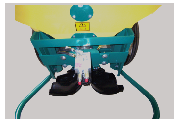
Variable speed hydraulic driven agitator & feed system
